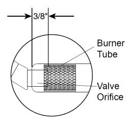
Burner tube must fit over valve orifice as shown.
